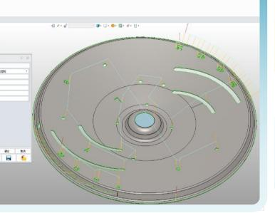
Uses processing solutions to quickly generate high-precision cutting trajectories, verify through physical processing simulation, import CL programs to convert into robot processing points, and optimize paths.
