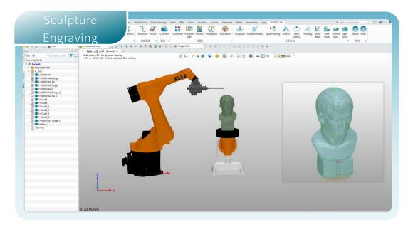
Rich robot trajectory processing algorithms quickly convert 5-axis and other machining trajectories into robot language, enabling comprehensive engraving trajectory planning.
