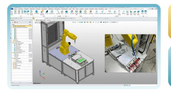
Visually simulates robot trajectory operation, real-time detection of path accessibility, singularity, and collision risks.
