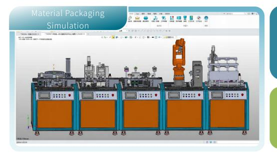
Material packaging simulation, including vibrating plates, multiple conveyor lines, robots, motor drives, material assembly, material transportation, and material warehousing
